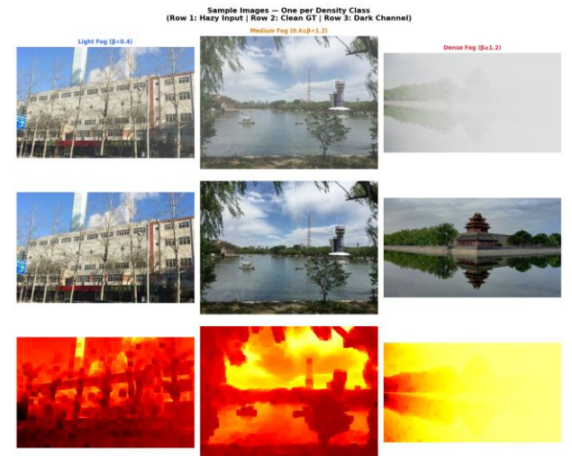
Fig. 2. Sample images at different fog densities, showing hazy inputs, ground truth, and dark channel priors.
