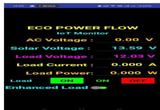
Fig 4: Case 1 – Normal Load (Working on Solar) a) mobile snapshot, b) model snapshot
