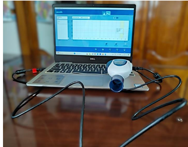
Fig 5. Connectivity of spirometer with computer and data transfer process
